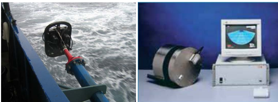
FIGURE 3.9. GeoAcoustics/Kongsberg GeoPulse sub-bottom profiler (left) and RESON SeaBat 8101 multibeam sonar (right, photo source: http://www.seafloorsystems.com ).
