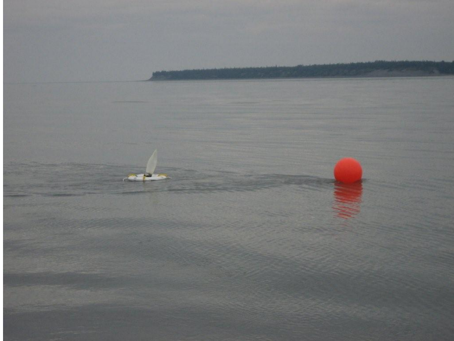
Figure 5. Omnidirectional sonobuoy (AN/SSQ-57B) deployed in Knik Arm with flotation ring and surface float.
