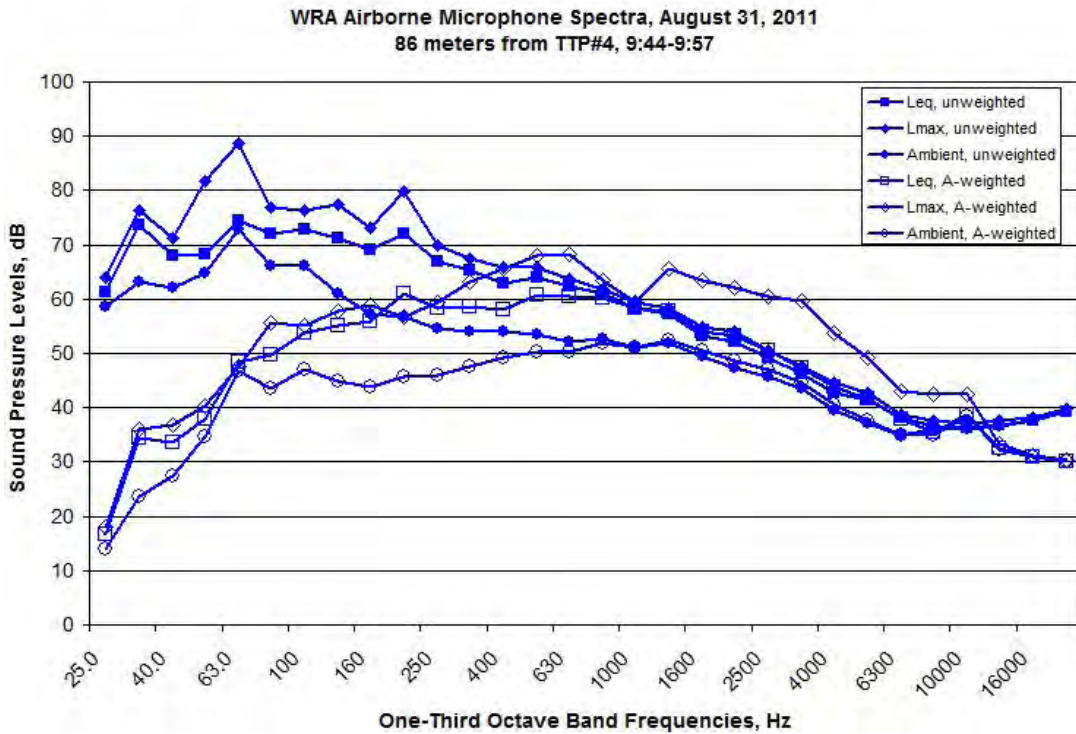
Figure C47. Average One-minute Unweighted and A-weighted Spectral Data Measured at the WRA Location during TTP#4, 9:44-9:57, on August 31, 2011
