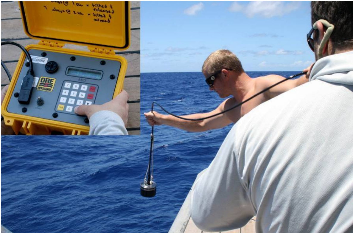
Figure 12. Communicating with EAR acoustic release to confirm deployment orientation and depth. Display at upper left reads a depth of “537 m”; vertical deployment orientation was also confirmed.
