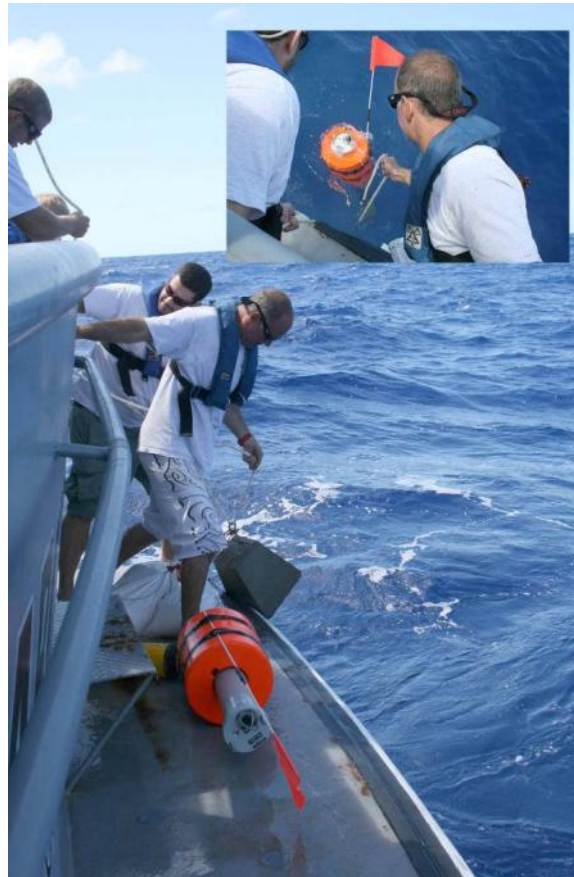
Figure 11. Deployment of EAR. The EAR is designed to be manually deployable without heavy equipment. Deployment location was 21^{\circ} 40.829'N 160^{\circ} 30.637'W at a depth of 537m. See Fig. 5 for location relative to Ka'ula.
