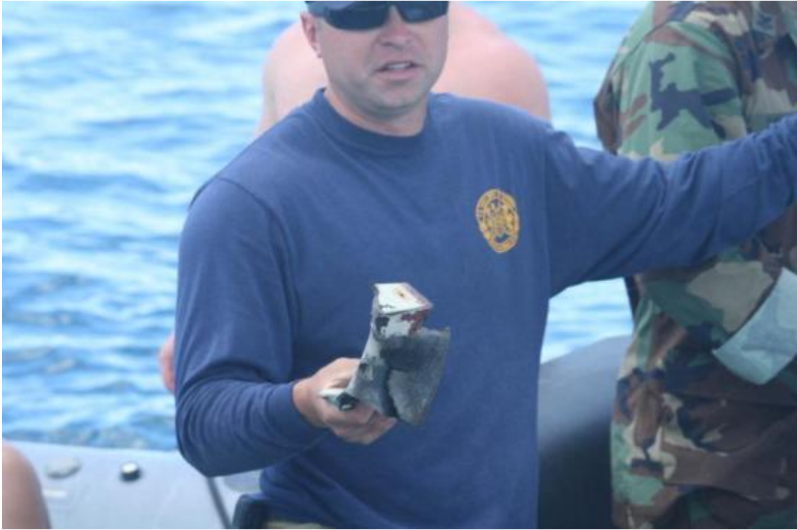
Figure 5. Sheared metal of the simulated obstruction after exercises of 26 April.
