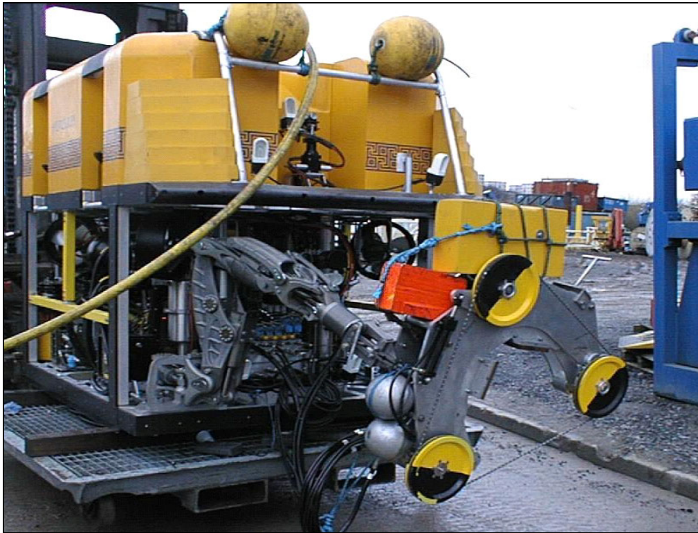
Figure 1-8. Diamond Wire Cutter Mounted to a ROV's Manipulator Arm (Courtesy of CUT USA, Inc.).
