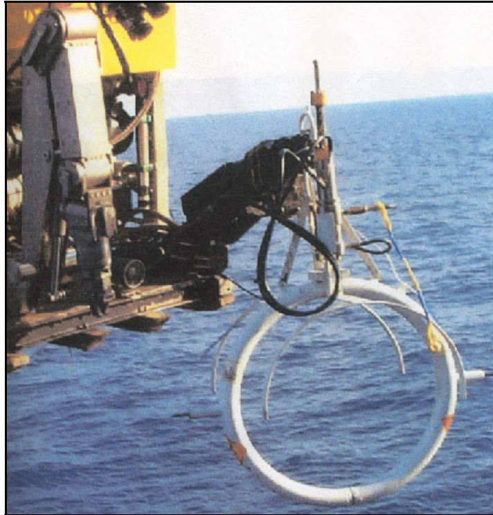
Figure 1-14. Externally-Deployed LSC Mounted to ROV (JRC, 2002).
