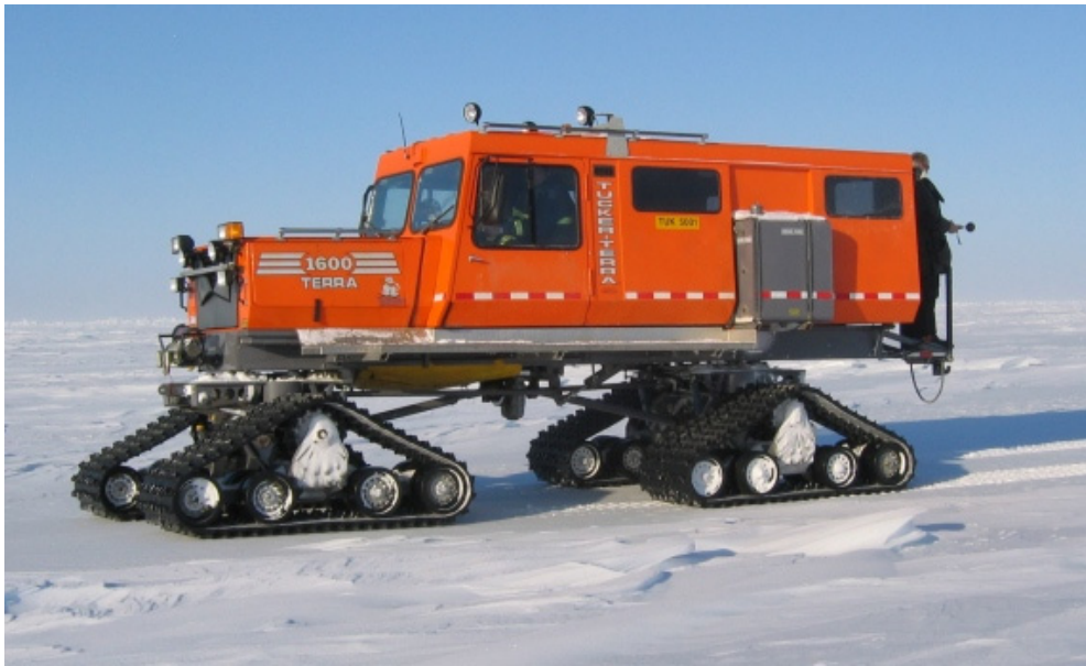
FIGURE 2.5. Tucker tracked vehicle used for transport of personnel during early winter and during spring break-up.
