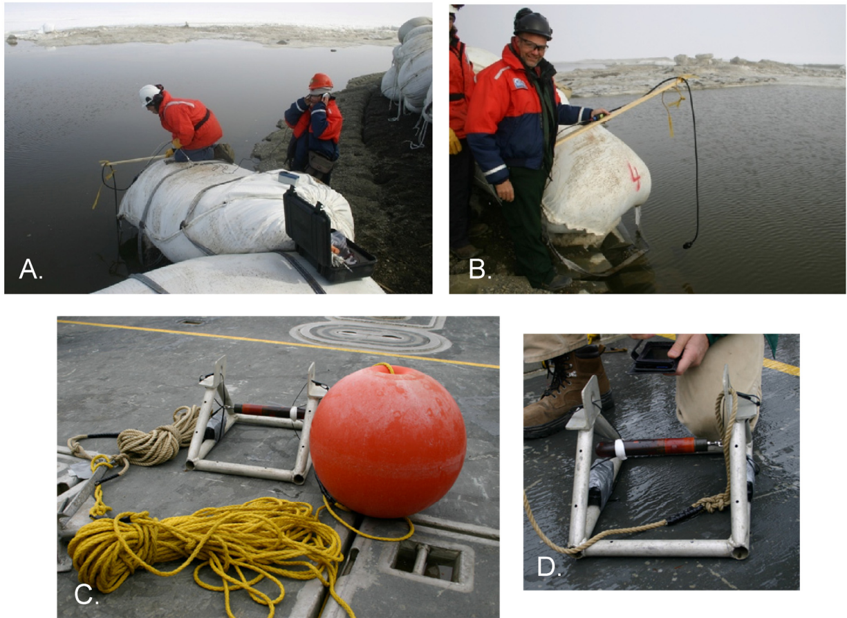
FIGURE 4.4: Pop sound investigation. (A) and (B) Listening for pops with a cabled hydrophone deployed in the moat along the western shore of Northstar, 11 June 2009. (C) and (D) Deployment of the Acousonde (the black and red cylinder within the metal stand) on 25 Aug. 2009. On that date, the Acousonde was deployed ~135 m northeast of the northeastern corner of Northstar and retrieved after ~ 7 hours.
