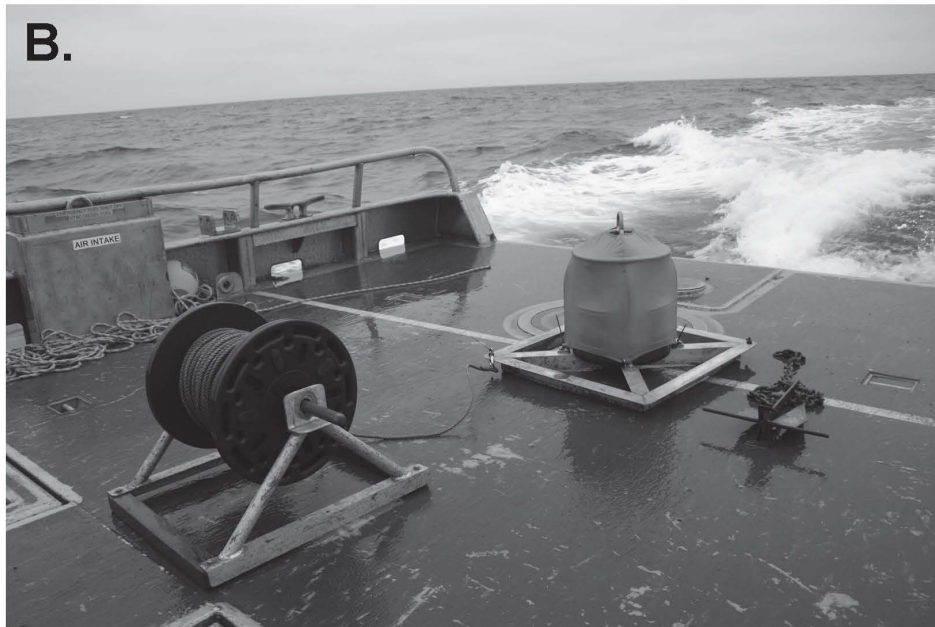
FIGURE 4.1. Directional Autonomous Seafloor Acoustic Recorder (DASAR). (A) Schematic diagram of the components of a DASAR (model C08) recorder. (B) A DASAR about to be deployed off the stern of an ACS Bay vessel. The ground line is on the reel (left) and the Danforth anchor and chain (right) are ready to be shackled to the ground line once the latter has been laid out on the seafloor. The DASAR is deployed first and the anchor last.
