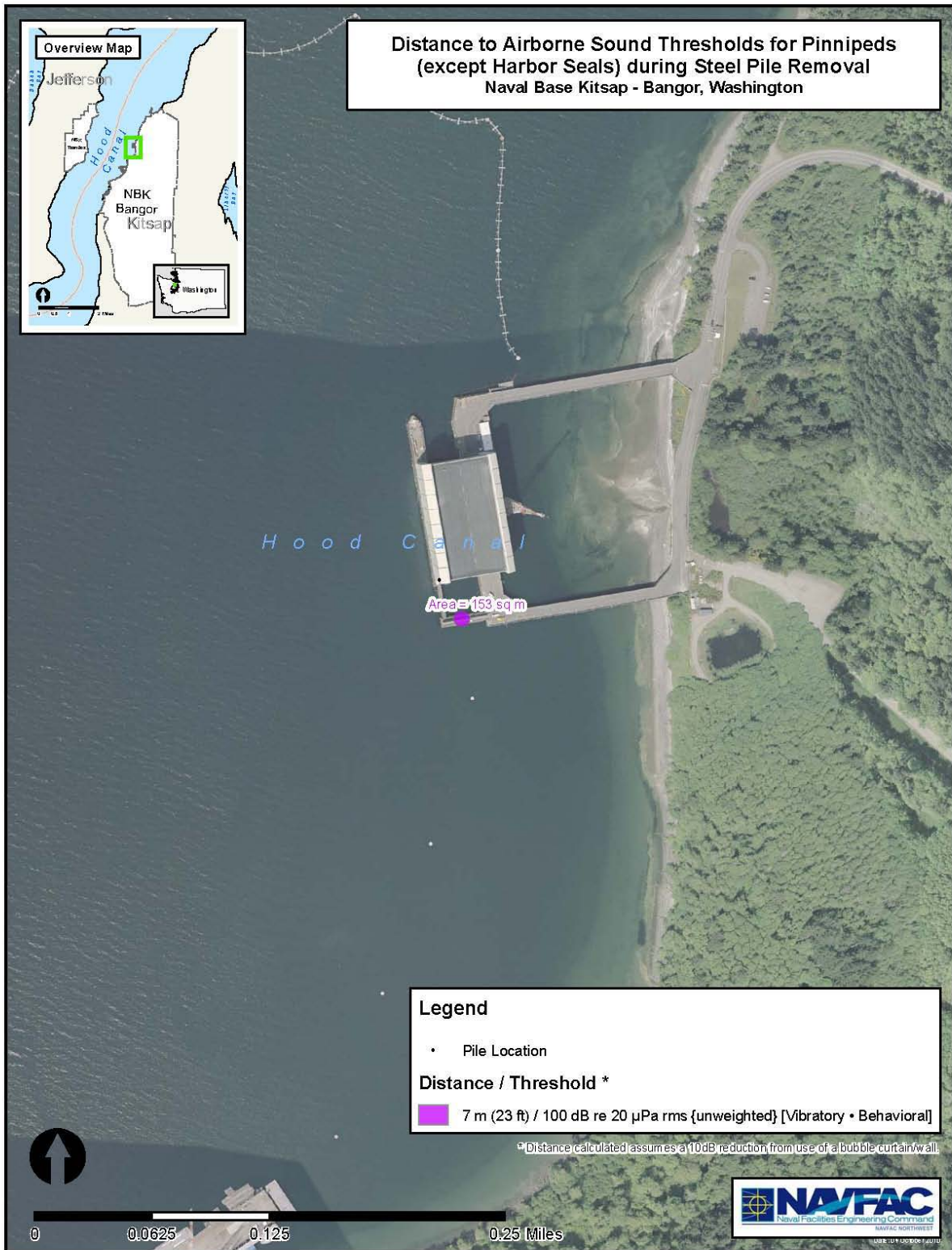
Figure 6-3. Distance(s) (m) to Airborne Sound Thresholds for Pinnipeds (except Harbor Seals) from Vibratory Steel Pile Extraction
