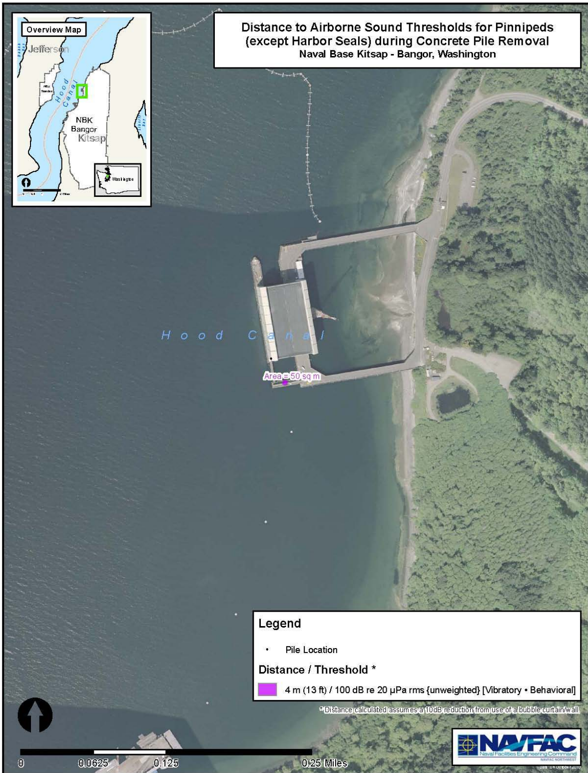
Figure 6-5. Distance(s) (m) to Airborne Sound Thresholds for Pinnipeds (except Harbor Seals) from a Chipping Hammer During Concrete Pile Removal
