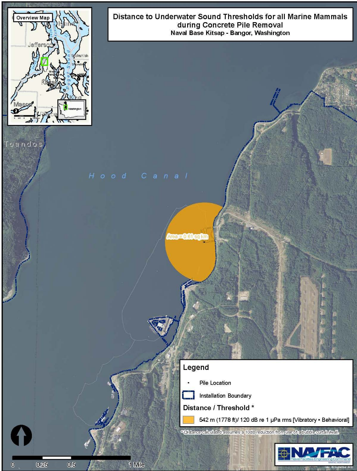
Figure 6-2. Distance(s) (m) to Underwater Sound Thresholds for all Marine Mammals from a Chipping Hammer During Concrete Pile Removal
