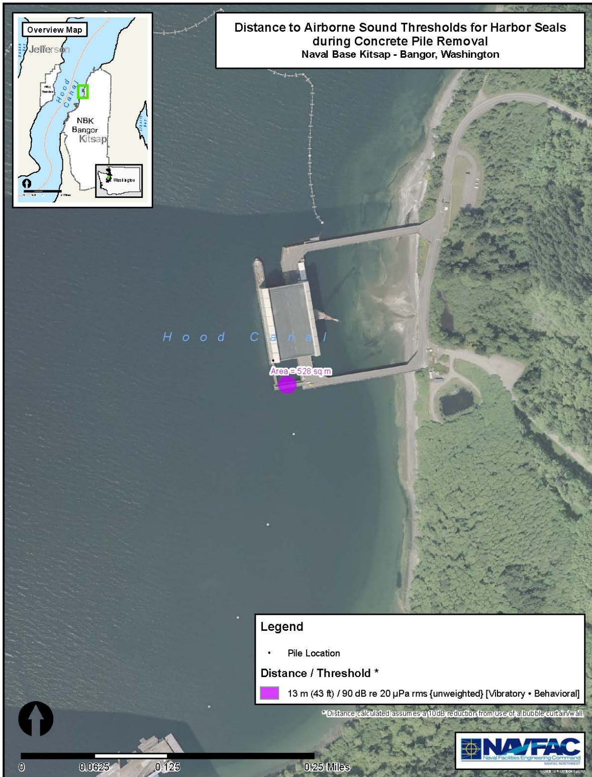
Figure 6-6. Distance(s) (m) to Airborne Sound Thresholds for Harbor Seals from a Chipping Hammer During Concrete Pile Removal
