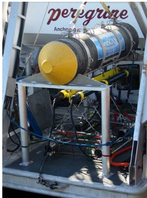
FIGURE 4.1 ONE 440 IN 3 AIRGUN ARRAY ON THE PEREGRINE.
