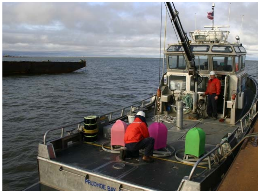
FIGURE 3.40 THE THREE DASARs USED FOR THE LIBERTY SEISMIC SURVEY ON THE ACS VESSEL GWYDYR BAY, JUST BEFORE THEIR DEPLOYMENT ON 3 AUGUST.
