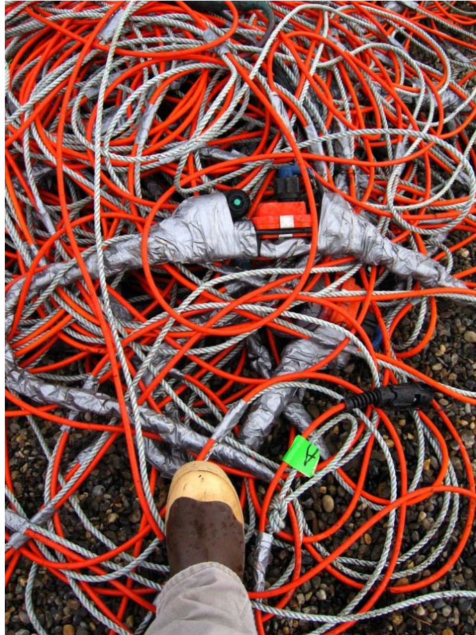
FIGURE 2.3 RECEIVER CABLES (ORANGE) WITH LEAD LINE, HYDROPHONE AND RECORDING UNIT USED DURING THE LIBERTY SURVEY.
