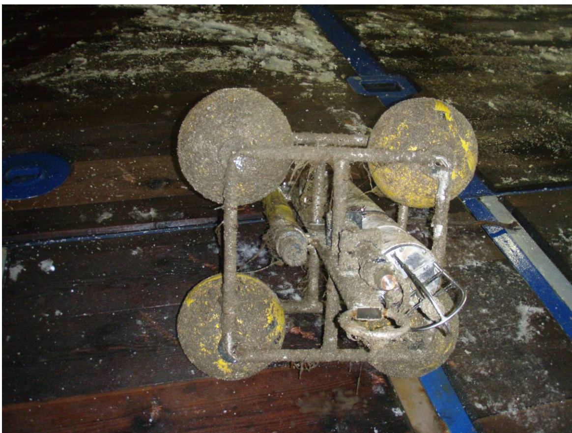
FIGURE 5.6. PL5 OBH with bio-fouling by barnacles.
