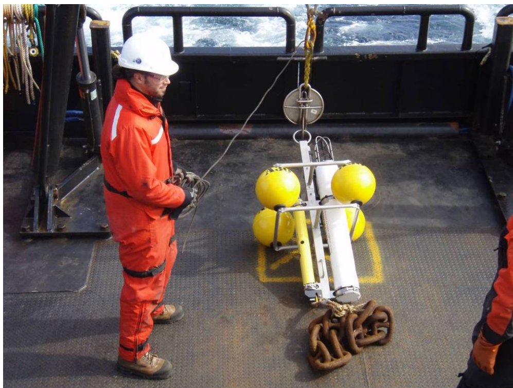
FIGURE 5.1. Ocean Bottom Hydrophone (OBH) system being deployed from the deck of the Norseman II during the 2007 Chukchi Sea acoustics study.
