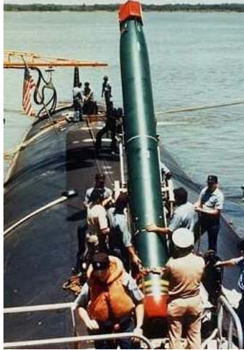
Figure 2-6. Depiction of MK-48 Torpedo Loaded onto Submarine
