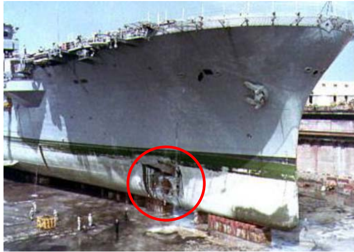
Figure 1-5. Depiction of Ship with Mine Damage
