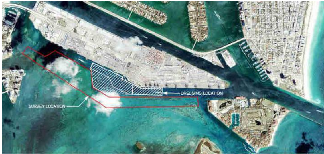
Figure 3 – (Figure 2 of the ACOE's IHA application) Blasting footprint for Phase II project.
