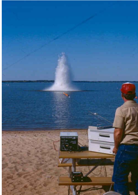
Figure 9 – (Figure 8 of the ACOE’s IHA application) Unconfined blast of 7 lbs of explosives.
