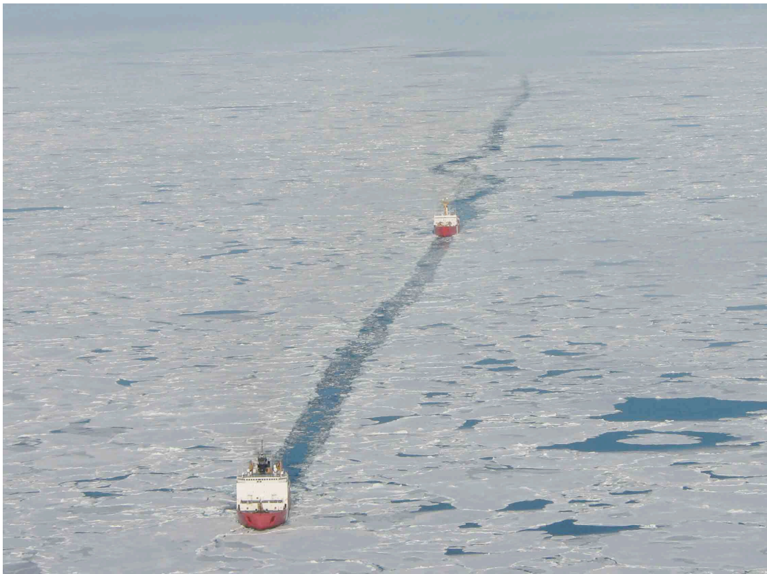
FIGURE J-1. Icebreakers Healy and Louis S. St. Laurent transiting 10/10 ice pack on 2 September 2009, showing minimal disturbance to the ice pack abeam of the ship's path, small jog to avoid larger ice body, and closing of the pack ice in the ship wake. (Photo courtesy of J. Biggar, DFO, Canada).
