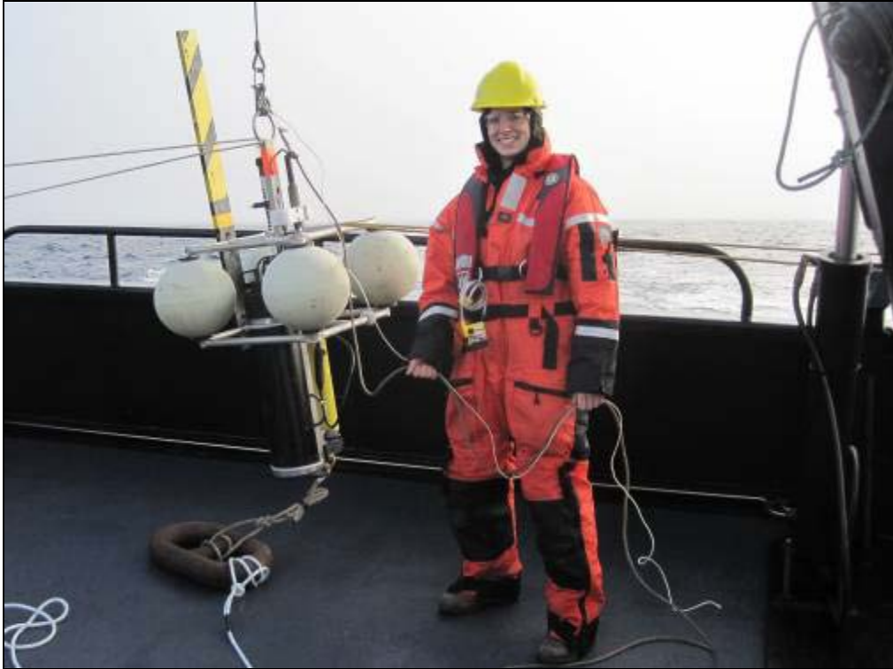
FIGURE 3.1. Photograph of a JASCO Ocean Bottom Hydrophone (OBH) recorder with ballast anchor.
