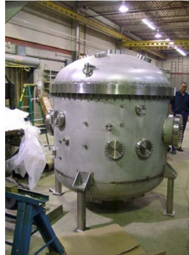
UHV vessel for Plasma Fusion experiment. Vessel is electropolished. Operates at 10^{-11} torr
