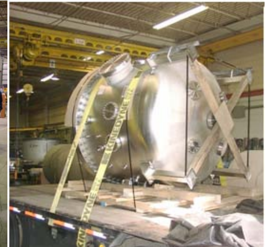
UHV vessel for Plasma Fusion experiment. Vessel is electropolished. Operates at 10^{-11} torr
