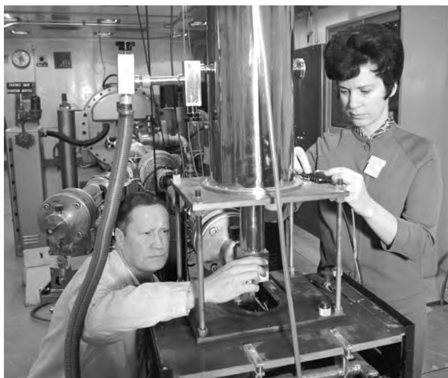
RUTH WHAN attaches thermocouple wires to monitor sample temperatures during irradiation on the Van de Graaff accelerator, while R. S. Neiman hooks up an electrical connection to monitor radiation levels.
