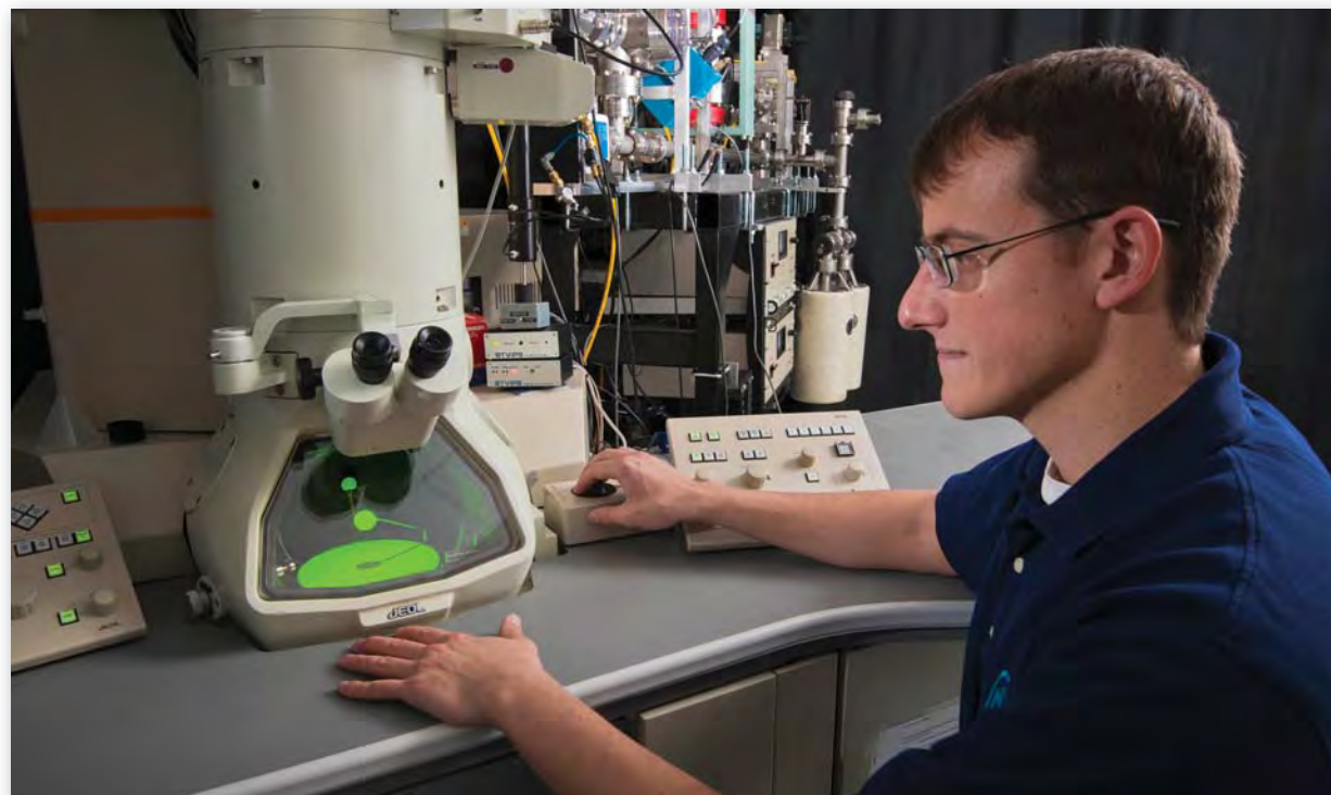
MATERIALS SCIENTIST KHALID HATTAR (1111) sits in front of the in situ ion irradiation TEM. The green light is electrons hitting phosphor. Khalid has been using Sandia's Ion Beam Laboratory for in situ ion irradiation experiments, potentially shaving years off testing new materials for nuclear reactors. (Photo by Randy Montoya)
