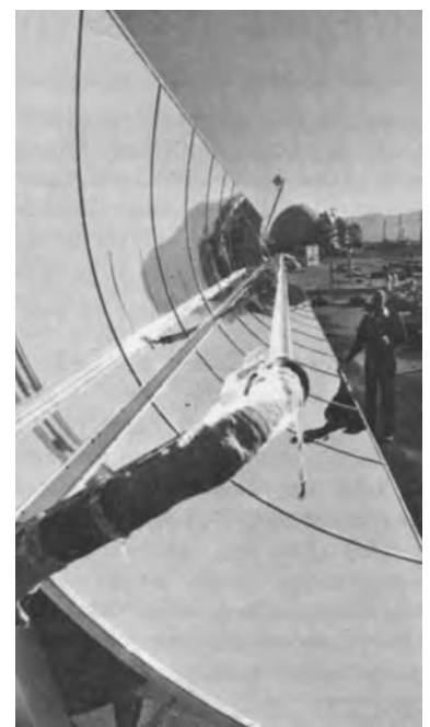
PARABOLIC TROUGH collector developed at Sandia offers highest efficiencies yet attained.
