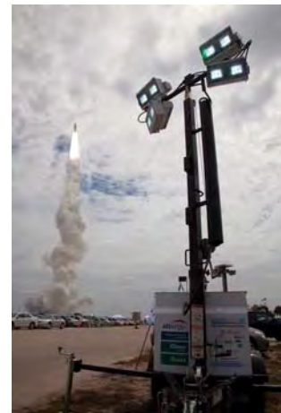
A FUEL CELL mobile light unit lit the grounds at the final space shuttle launch at the Kennedy Space Center in July 2011.
