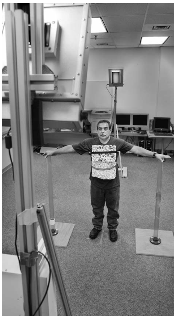
SCAN MAN — The Concealed Threat Detector scans a subject suspected of wearing an explosive device.
