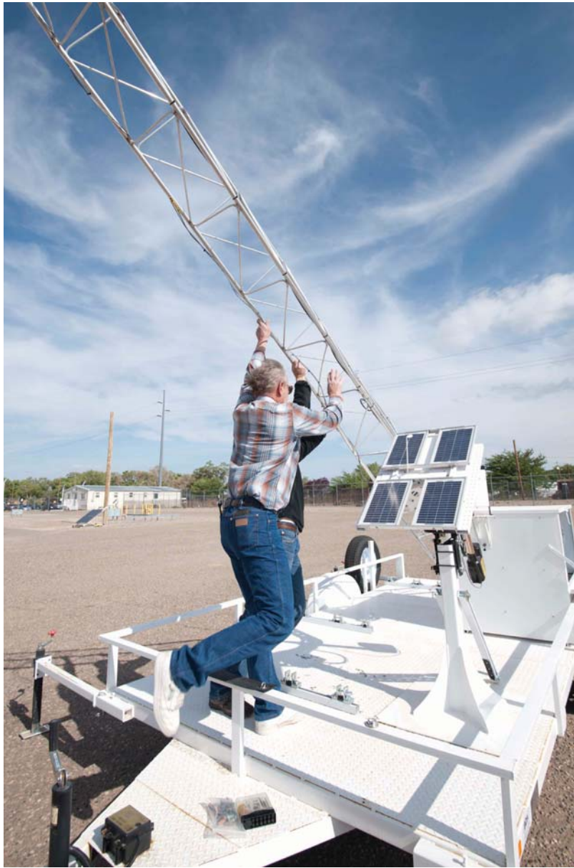
PRECISION SOLAR TECHNOLOGIES owner Tim Leonard, foreground, and the company's project engineer, Tony Louderbough, hoist a mast that is part of the company's Prospector Mule trailer-mounted solar weather station. Precision Solar uses a tracking technology developed at Sandia as an integral part of the weather station. (Photo by Randy Montoya)
