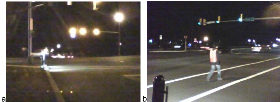
Figure 24. a) View toward crosswalk from Texas Road, showing the light pattern along the crosswalk; b) view of pedestrian crossing the road, showing the relatively high vertical illuminances
