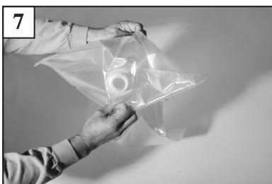
Remove cap from bag. Pull bag sides apart to allow liquids to fill.
