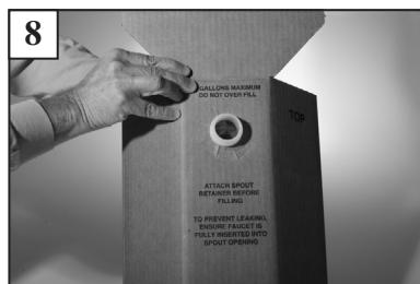
From inside box, insert spout through cutout of box wall.
