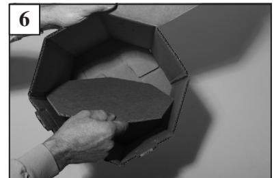
Place reinforcement disk in bottom of box.
