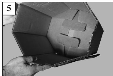
Turn box over so bottom faces downward. Push down tabs to form flat bottom.
