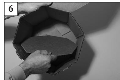
Place reinforcement disk in bottom of box.
