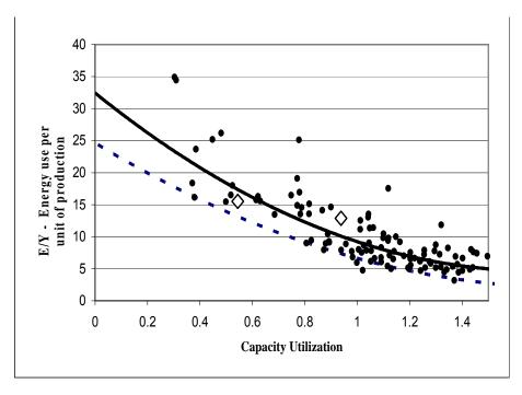
Figure 1 COLS and Frontier Regression of Energy Use per Unit of Production against Capacity Utilization
