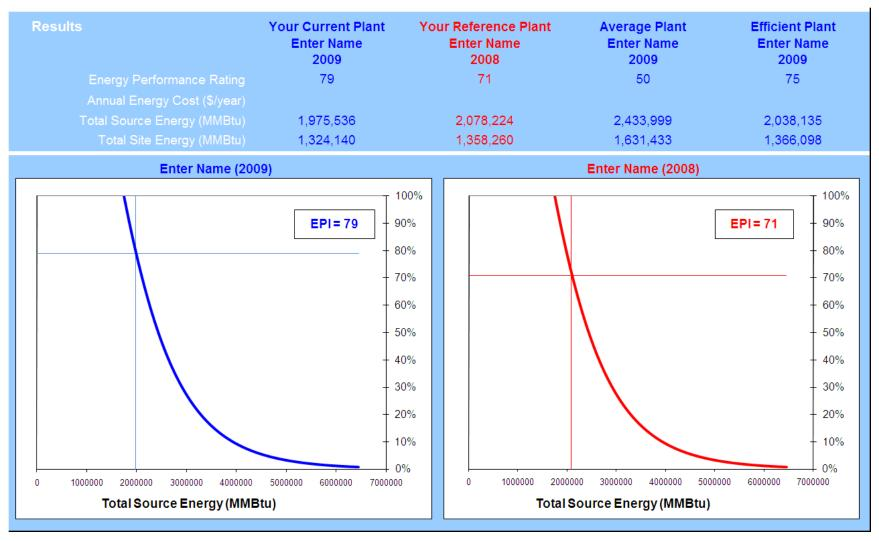
Figure 5 Output Section of the Flat Glass EPI Spreadsheet Tool
