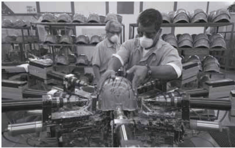
A Beaumont inmate drills a Kevlar helmet to specification for hardware attachment.
