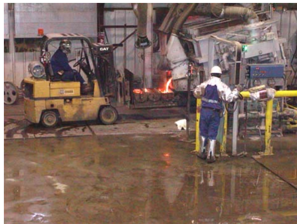
Figure 2. Operation with housekeeping and remote furnace controls
