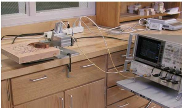
Microwave moisture measurement system for lumber drying.
