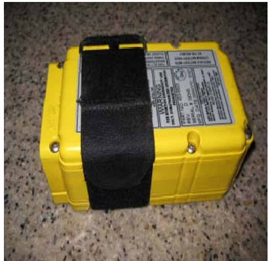
Figure 2. Artex ME406 ELT and separate mounting tray (left); ELT in mounting tray, secured by Velcro strap (right).
