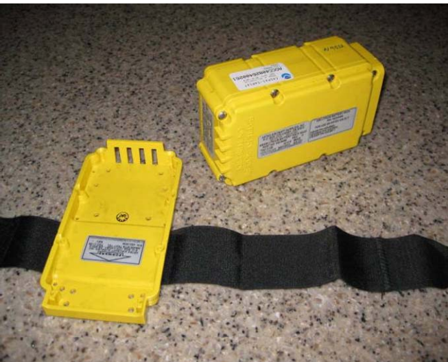
Figure 2. Artex ME406 ELT and separate mounting tray (left); ELT in mounting tray, secured by Velcro strap (right).
