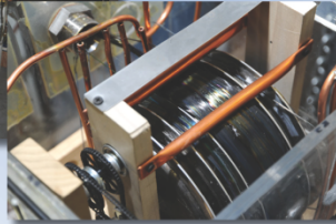
Figure 6: INL's SiC Direct has produced \alpha -SiC fibers in continuous coiled form with lengths up to a mile (e.g. 1,800 meters) or longer.
