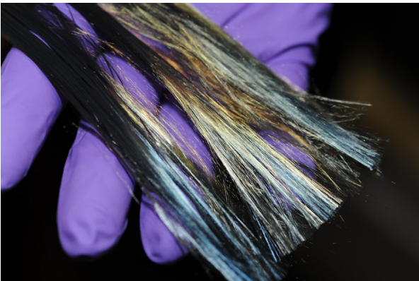
\alpha -SiC/C fiber have been converted from 50,000 and 3,000 filament carbon tows. These fibers have color from irradient green, purple to blue as a result of light scattering from sub-micron SiC grains and residual elements, such as N 2 (green).
