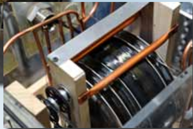
Figure 6: INL's SiC Direct has produced \alpha -SiC fibers in continuous coiled form with lengths up to a mile (e.g. 1,800 meters) or longer.
