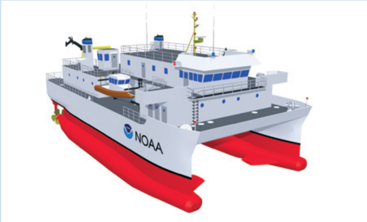
NOAA will replace RUDE with a new coastal mapping vessel. Shown is an artist's rendering of the newly designed Small Waterplane Area Twin Hull (SWATH) vessel.
