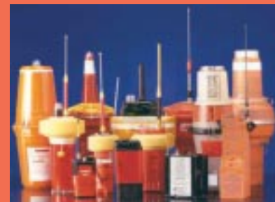
Emergency beacons used in the COSPAS-SARSAT search-and-rescue system.
