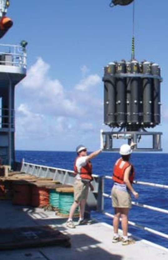
Ocean Exploration scientists launch the CTD, (“conductivity, temperature, depth”) over the side of the research vessel THOMPSON to take ocean measurements.
