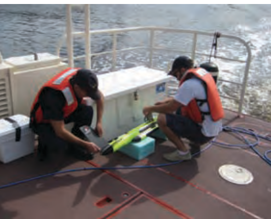
Following Hurricane Ike, NOS used the NOAA Mobile Integrated Survey System to search for hazards to navigation.
