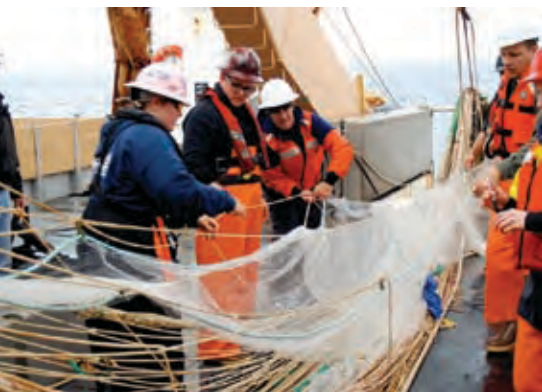
Crew members attach pocket nets to test whether the Aleutian wing trawl is an accurate sampling tool for determining how many fish can escape the net during a trawl. Photo: Mark Rauzon, U.S. Fish and Wildlife Service
