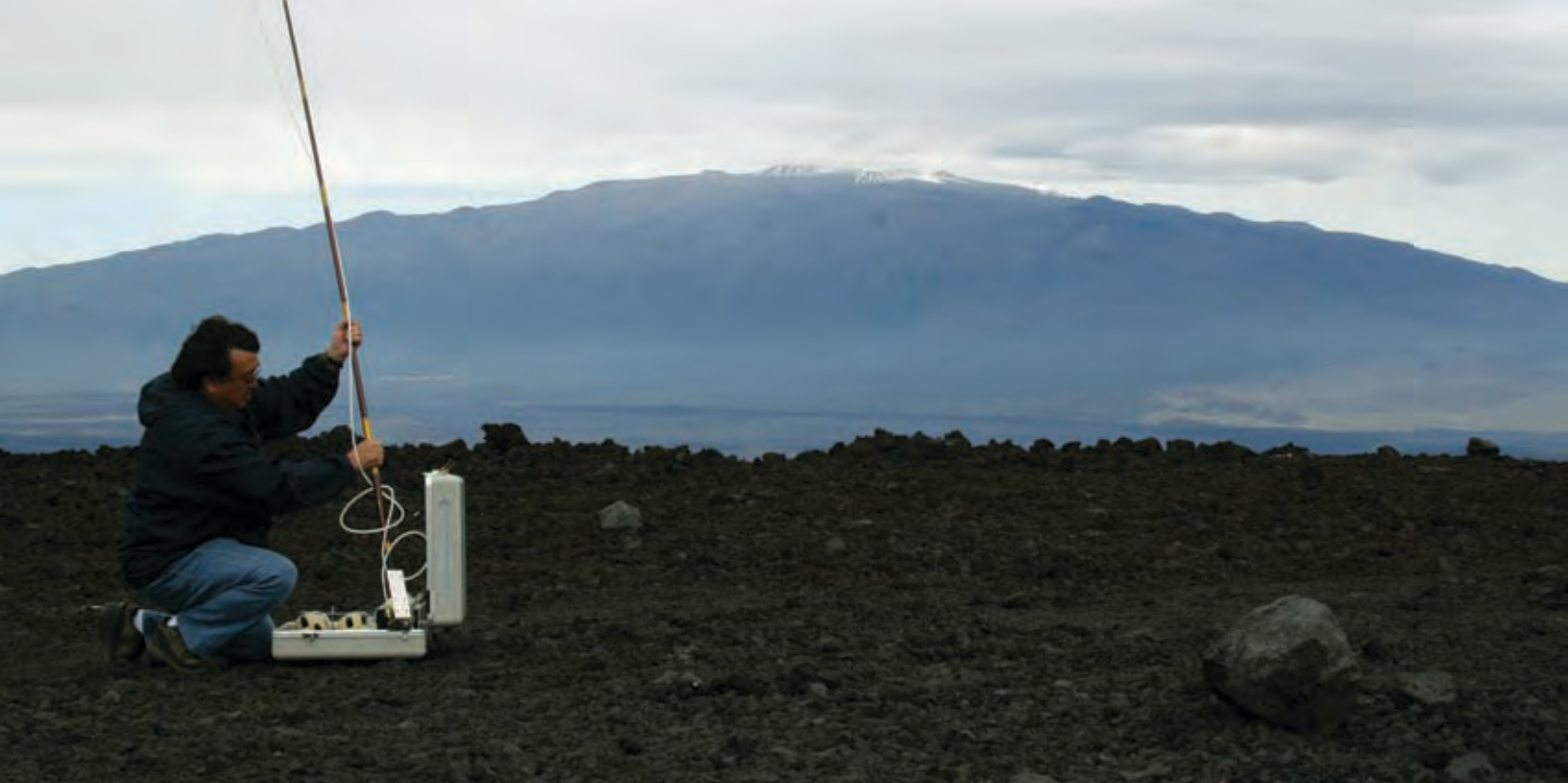
NOAA engineer Paul Fukumura-Sawada captures air near NOAA's Mauna Loa Observatory in Hawaii, using one of many methods to measure carbon dioxide and other greenhouse gases in Earth's atmosphere.
