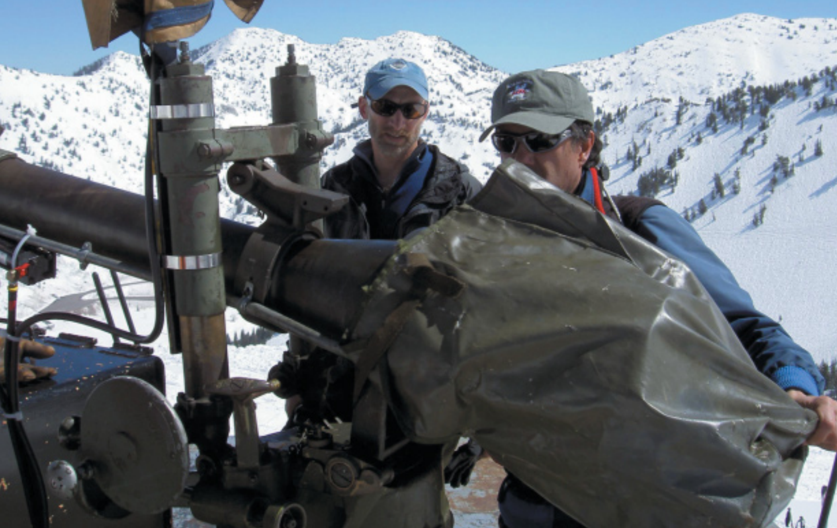
Gabe Garcia, a snow safety official at Alta Ski Area, unveils a 105-millimeter recoilless gun used for avalanche control in Little Cottonwood Canyon to Meteorologist-in-Charge Larry Dunn, of the Weather Forecast Office (WFO) in Salt Lake City, Utah. Officials from the ski areas and Utah Department of Transportation work closely with the WFO, the Forecast Service Utah Avalanche Center, and local communities to help keep recreationers in the canyon safe. Snow accumulations approaching 700 inches in parts of the canyon made 2004–2005 an especially challenging season. Photo: Kevin Barjenbruch, WFO Salt Lake City
