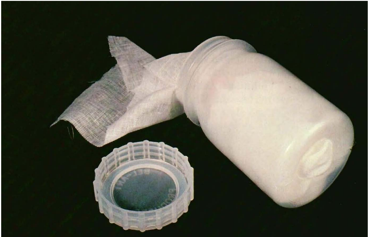
Figure V-3. The Spira swab is used for filtering large volumes of water through cotton gauze to recover V. cholerae
