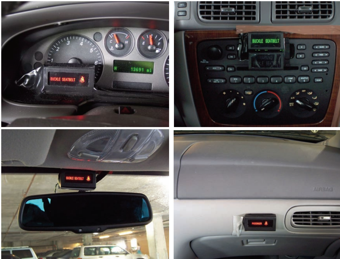
Figure 1. Seat belt reminder displays (clockwise from top left: dashboard display, center console display, passenger display, rear view mirror display)
