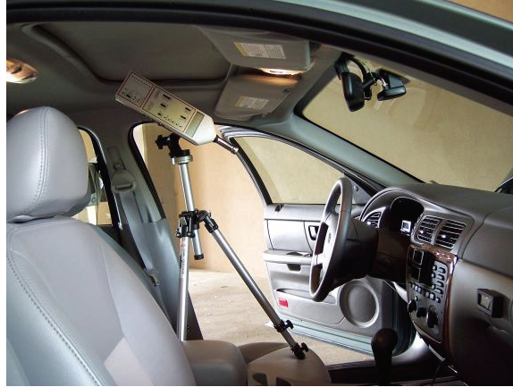
Figure 2. Sound level meter positioned on driver's seat
