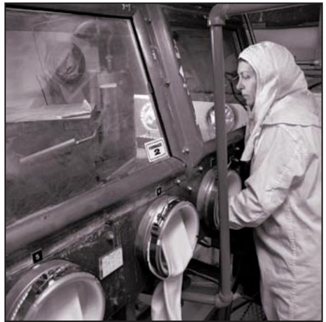
Small ovens, called muffle furnaces, dry small batches of plutonium-bearing materials, converting them to a more stable form. Hanford will use this thermal process to stabilize three-quarters of PFP's 4.3 metric tons of plutonium.
