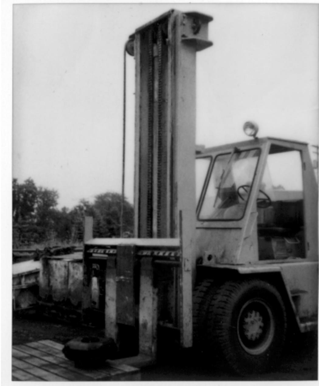
**Figure.** Fork Truck Components: 1) fork carriage (assembly to which the forks or other attachments are mounted, and 2) mast (steel upright assembly consisting of hydraulic cylinders, inner channels, telescoping outer channels, chains, and guide rollers).
