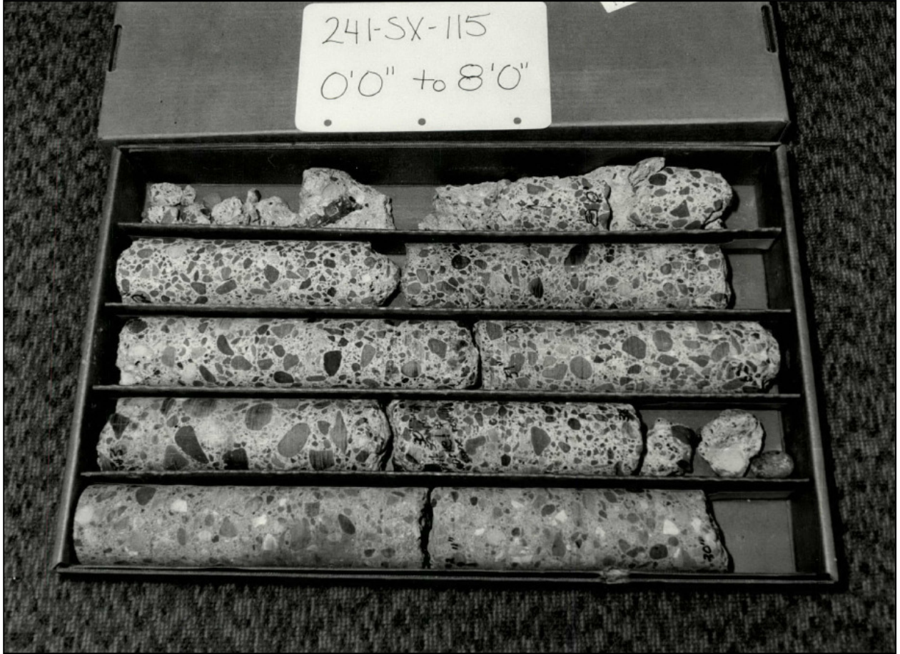
Figure B-6: Photo of Cores Pulled From 241-SX-115
