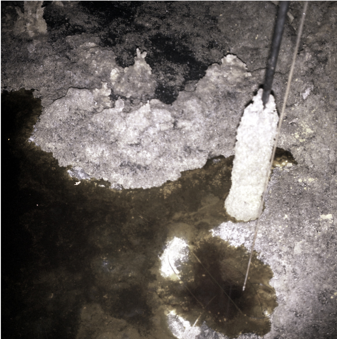
Figure B4-11. Salt Crystals on Tank 241-BX-110 Manual Tape (January 31, 1974)
