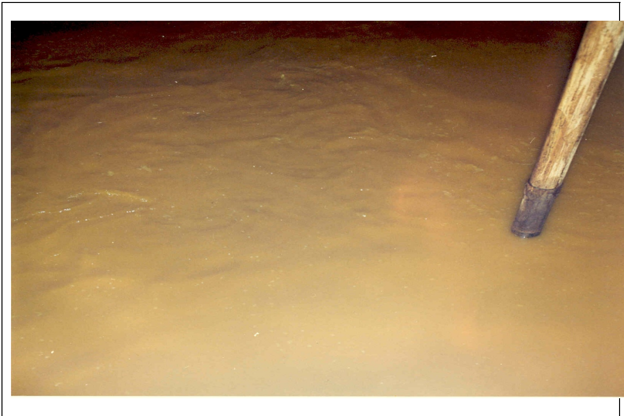
Figure 4-1. Tank SX-110 Surface Condition Typical of Air-Lift Circulator Effects, June, 1974
