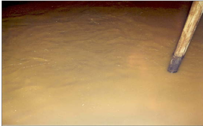
Surface chop resulting from airlift circulator operation.
