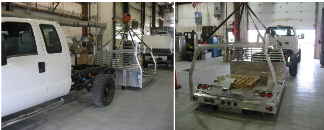
Assembling new flatbed truck for Electrical Utilities
