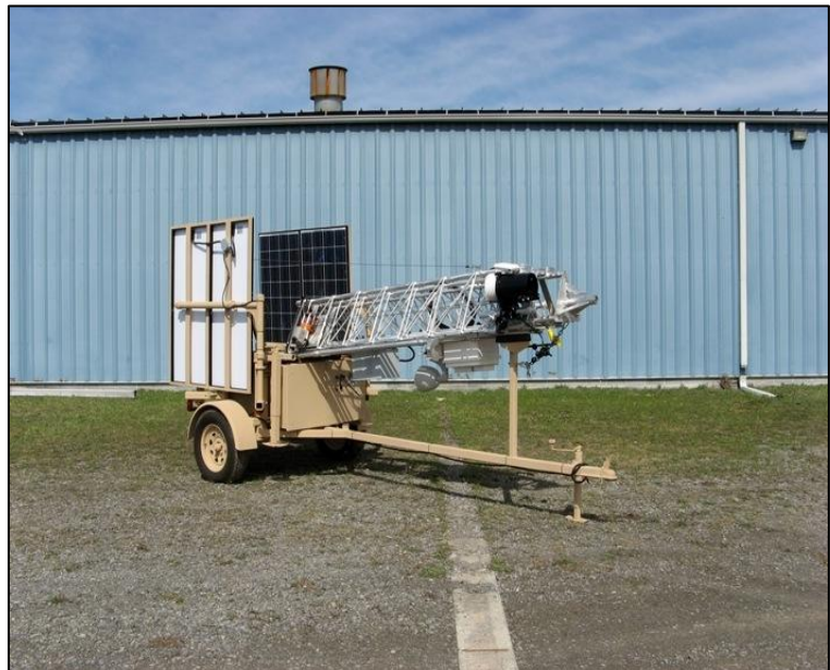
Wireless Wind and Solar Powered Platform – portable unit that provides voice, video, or data services
