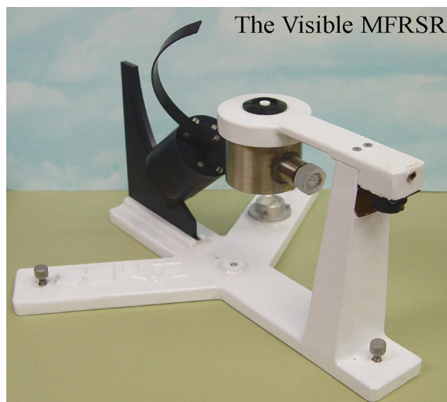
Figure 1. The visible MFRSR. This particular unit is a Yankee Environmental Systems, Inc. model.
