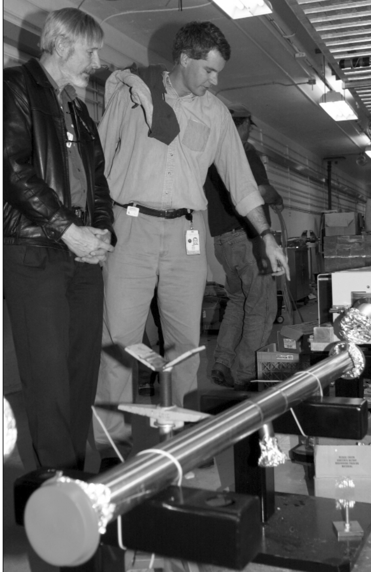
Lab Director Christoph Leemann (left) accompanies Will Oren, Accelerator Engineering Dept. head, on an accelerator safety walk through during the recent maintenance period. Here they examine a segment of the energy recovery experiment beamline under assembly.
