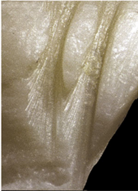
Figure III-35. False start: flare at one end. This suggests the end of the kerf where flexible saw blade is flared due to lateral movement of the handle, while the blade supported by the kerf does not flare.
