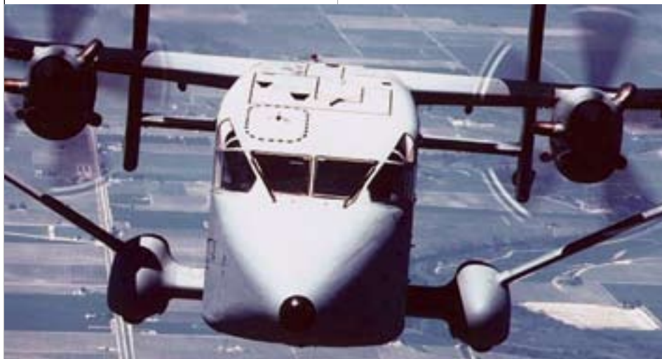
ABOVE: The C-23B Sherpa, designed for Short Take-off & Landing (STOL), can hold 30 troops and operate from unpaved runways.
