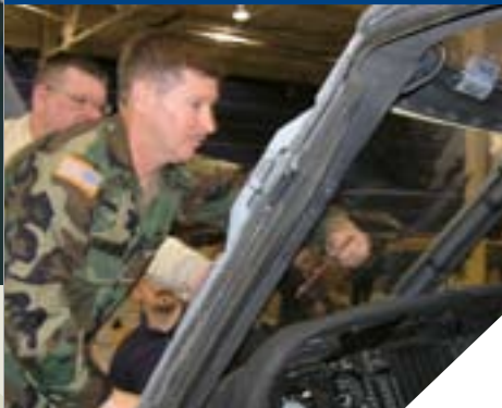
LEFT: SFC Paul Kagi, a helicopter mechanic assigned to the 2nd Bn., 224th Aviation Regt., VAARNG, applies a DSCR-developed laminate to the windshield of a UH-60 Black Hawk helicopter at the Feb. 22 demonstration. Photo by Will Daniel
