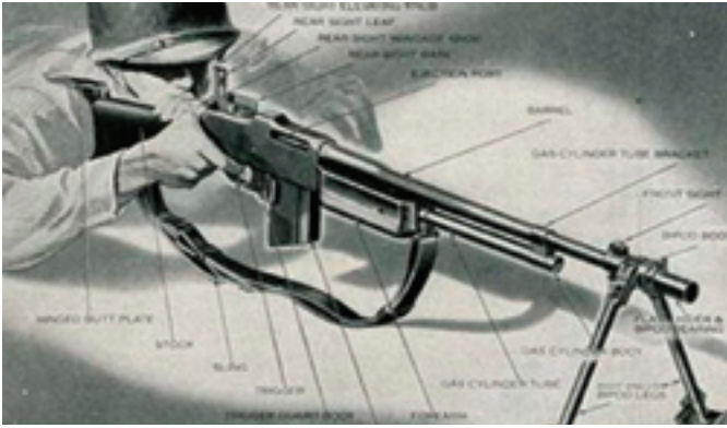
GETTING TECHNICAL An illustration that appeared in early military training manuals, outlining the BAR's basic parts.
