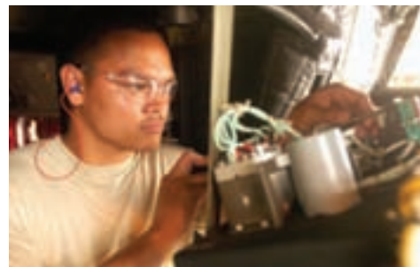
SWITCH ON SPC Gabby Balicoco, aircraft electrician with the 777th Aviation Support Battalion, Hawaii Army National Guard, attaches a new loading ramp lowering switch to the control panel of a CH-47 Chinook helicopter.
