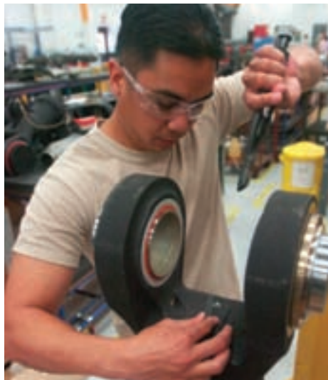
TOOLS OF THE TRADE SSG Jarrett Cummings, aircraft power train repair technician, attaches a safety wire to the main rotor head-unit of a UH-60 Black Hawk during the 777th's Annual Training mission.
