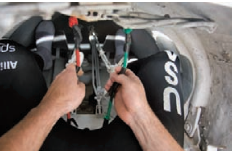
STEERING SYSTEM A bobsled is steered by two D rings attached to a rope and pulley system that connects to the front runners. If you pull the right ring you turn right and vice versa.
