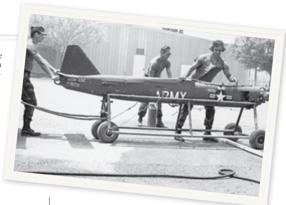
REMOTE CONTROLLED BOMBER Members of the 200th Air Defense Artillery Detachment wheel out a Radio Controlled Aerial Target (RCAT) on the White Sands Firing Range, NM.
