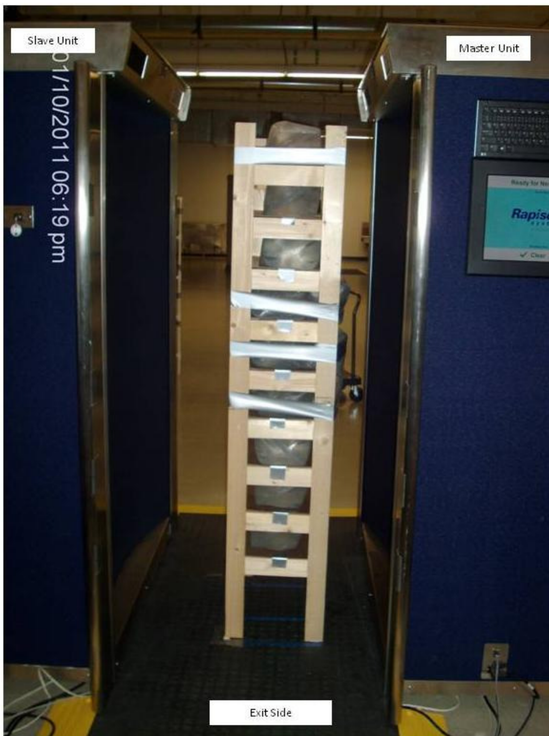
Figure C.1. Water phantom positioned inside the Secure 1000 SP.
