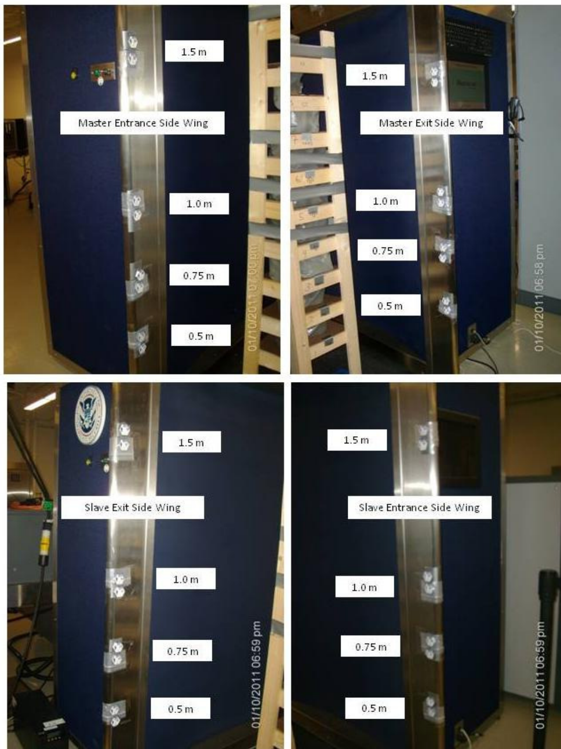
Figure E.1. Arrangement of dosimeters on wings
