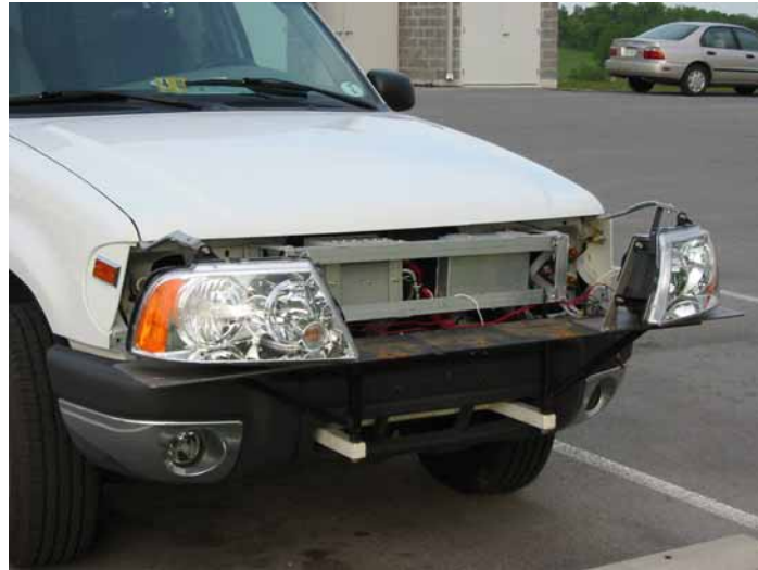
Figure 24. Photo. Headlamp testing rack.
