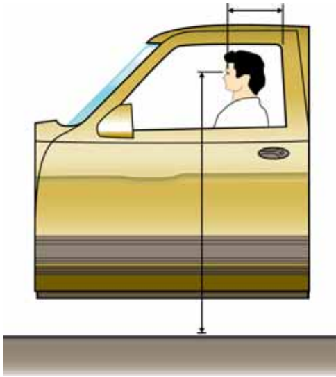
Figure 85. Diagram. Eye position measurement locations for all experimental vehicles (forward measure taken from leading edge of B-pillar weather seal).
