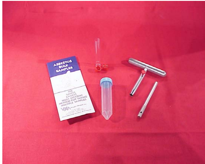
Figure 8-3. Bulk/Core Asbestos Sampler/Container
