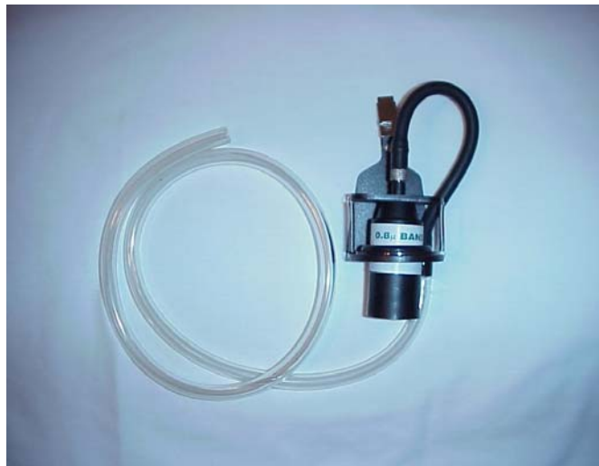
Figure 8-2a. Alternate Asbestos Fiber Sampler
