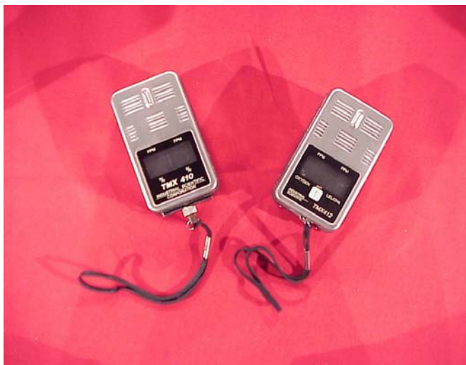
Figure 13A-1. Industrial Scientific Corporation Models TMX – 410 and TMX – 412
